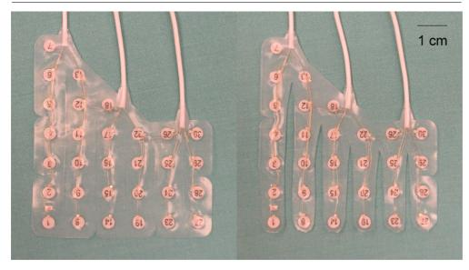
Figure 1. 30-contact TP grid before and after cutting columns (left and right panel, respectively).
