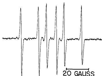
Fig. 4. An example of the alpha-hydroxyethyl radical spin adduct of DMPO ( a_N = 15.8 gauss, a_H = 22.8 gauss). This reaction mixture was the same as Fig. 3 except ethyl alcohol was included at 1 M. The gain was decreased by a factor of three, and all other instrument settings were the same as in Fig. 3. The same spectrum is observed if the ethyl alcohol concentration is reduced to 0.1 M, except there is also a small amount of DMPO/OH signal present in the spectrum
