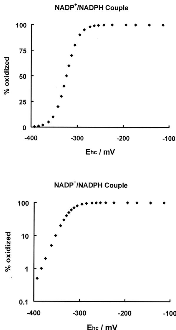
Fig. 2. The reduction potential of the  $\text{NADP}^+/\text{NADPH}$  half-cell becomes more positive with increasing  $\text{NADP}^+$ . The midpoint potential of this couple is taken as  $-315$  mV at  $25^\circ\text{C}$  and pH 7.0. The linear and log plots provide quite different perspectives on the behavior of this redox pair. Data points are derived from calculations using Eqn. 19.
