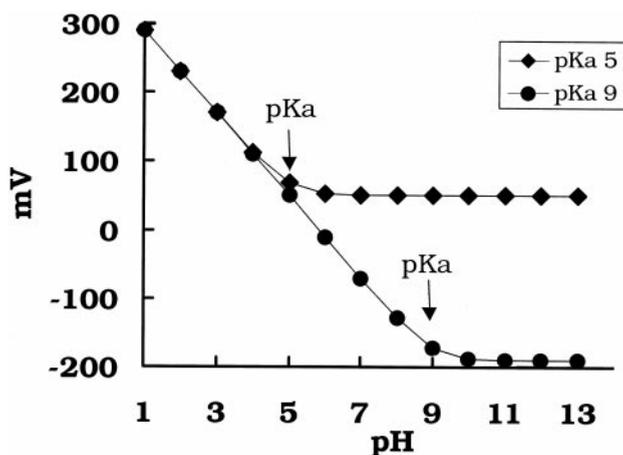
Fig. 1. The reduction potential of redox couples can be pH dependent. Shown are two examples of how the reduction of two different redox pairs change versus pH. The two examples have quite different  $pK_a$ s, but the half-cell potentials at  $pH = 0$  are the same. Data were derived from Eqn. 10 using a half-cell potential of +350 mV at  $pH = 0$ .
