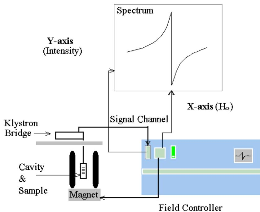
Figure 2. The general outlay of an EPR spectrometer.
